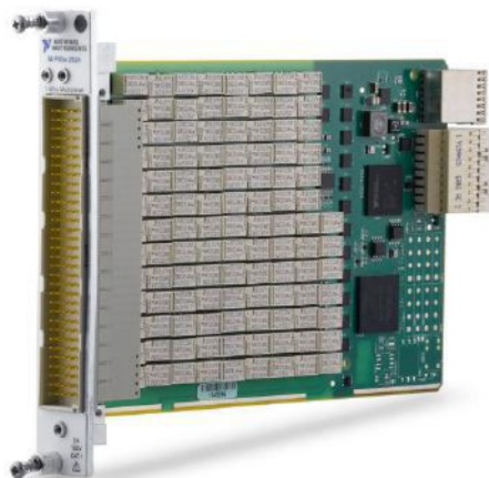
Figure 3. The PXIe-2524 is one example of a PXI Multiplexer Switch Module that can be reconfigured into various multiplexer topologies, ranging from 16 independent 8-channel multiplexers to a single 128-channel multiplexer.
